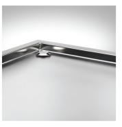
As an option, for harsher environments, we also offer a special anti-fingerprint finish: the 316 stainless steel surfaces first undergo a special micro shot-peening treatment and are then electropolished to create a bright, silk-smooth surface that doesn't compromise on cleanability or esthetics.
