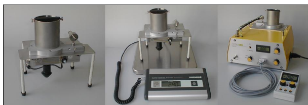
Optional accessories for the basic device: Dispersing unit SAG 410 (left), Dispersing unit on a scale for Online-Measurement (middle), SAG 410 with remote control (right)
