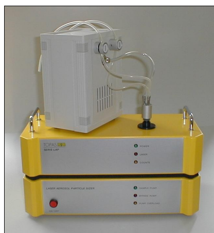
LAP 322 with Sample Switching Unit SYS 520
