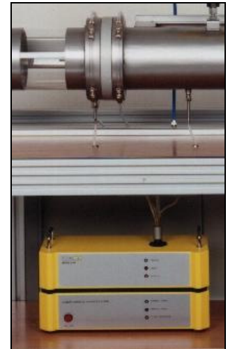
Straightforward investigation of the fractional collection efficiency in dependence on the load in the raw gas (setup including a SYS 520 switching unit below a Topas filter testing channel AFC 131)
