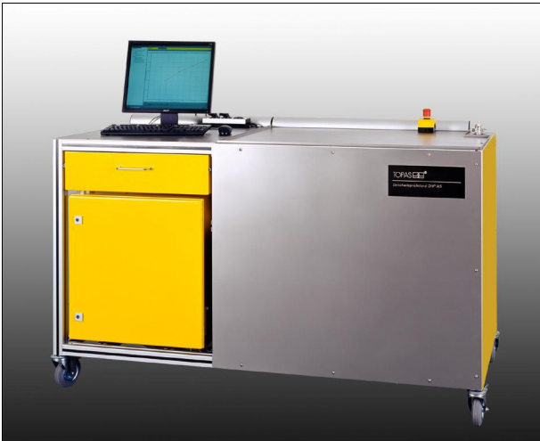
Test Rig for Leak Test DHP 145
