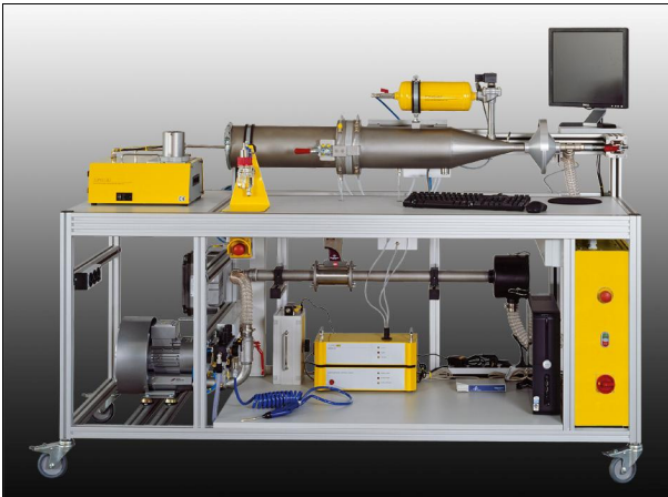
Filter test rig AFC 131 according to VDI 3926 Part 1, version 2
