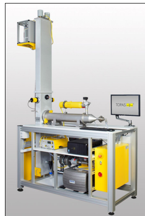
Filter test rig AFC 133 per as ISO 11057, VDI 3926 Part 1, version 1
